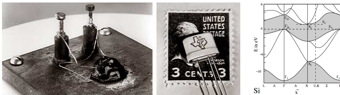
Figure: (Left) First silicon transistor (Bell Labs, Murray Hill, NJ) announced in 1951 by William Shockley; (Right) Silicon band structure. Shaded area indicates energy domains with no allowed states.
